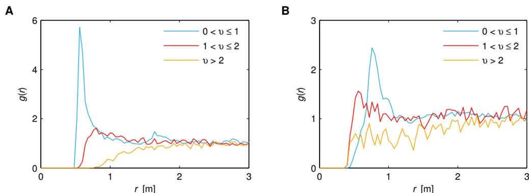
FIG. S5. The pair distribution function  $g(r)$  in the hallway simulation generated using (A) the interaction force described in Eq. (S2), and (B) the distance-dependent force described in [11]. The variable  $v$  denotes the rate of approach between pedestrians, and is measured in units of m/s. See also Fig. 1c of the main text.
