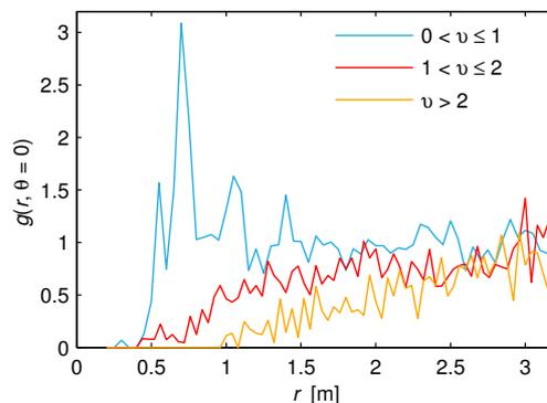
FIG. S2. The pair distribution function  $g$  in polar coordinates  $(r, \theta)$  for pedestrians in the *Outdoor* dataset, plotted for the fixed angle  $\theta = 0$ .  $g(r, \theta = 0)$  shows a significant dependence on the rate  $v$  at which the pedestrians approach each other, indicating that the displacement vector  $\mathbf{r}$  is not a sufficient descriptor of pedestrian interactions.
