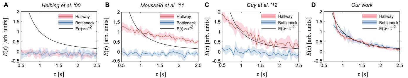
FIG. S6. The inferred interaction energy  $E(\tau) \propto \ln(1/g(\tau))$  as a function of time-to-collision ( $\tau$ ) for simulations obtained using (A) the distance-dependent model described in [11], (B) the behavioral heuristics model proposed in [16], (C) the least-effort model proposed in [15], and (D) our derived anticipatory force model. In all figures, colored lines indicate average energy values every 0.05 s and shaded regions denote  $\pm$  one standard deviation.
